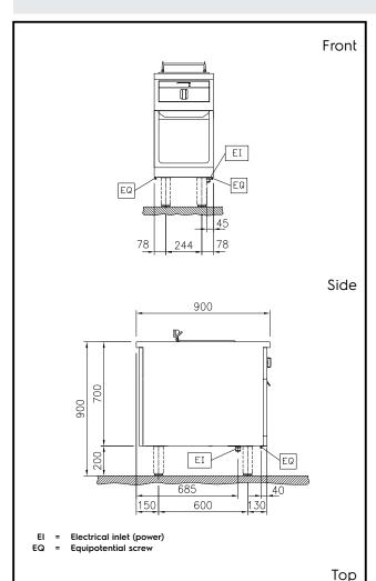
Electric Supply voltage: 400 V/3N ph/50/60 Hz Total Watts: 5.4 kW **Key Information:** Number of wells: Usable well dimensions (width): 240 mm Usable well dimensions (height): 135 mm Usable well dimensions 380 mm (depth): Well capacity: 6 lt MIN; 7 lt MAX Thermostat Range: 100 °C MIN; 180 °C MAX External dimensions, Width: 400 mm External dimensions, Depth: 900 mm External dimensions, Height: 700 mm Net weight: 70 kg
